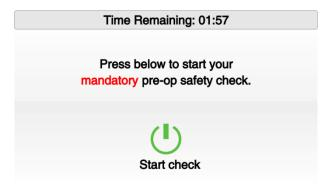
Note: If your vehicle has a speed controller and the Fleet IQ LCD is configured to use it, the vehicle will be in slow-mode when completing the PreOp check. Once the PreOp check is completed, the vehicle will be switched to normal operation.
